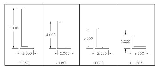
NOTE: SINGLE FLANGE ANGLES ARE PRIMARILY USED FOR MULTIPLE SECTION LOUVERS ADJACENT TO SECTION BREAK LOCATIONS.
