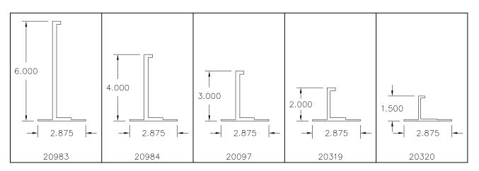
NOTE: DOUBLE FLANGE ANGLES ARE USED AT INTERMEDIATE SUPPORT LOCATIONS AND CANNOT BE USED ADJACENT TO SECTION BREAK LOCATIONS.
